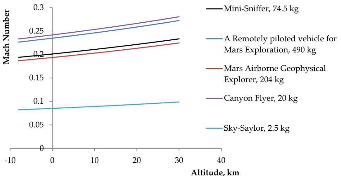
Figure 3. Cruising Mach number vs flight altitude for existing Mars aircraft projects
